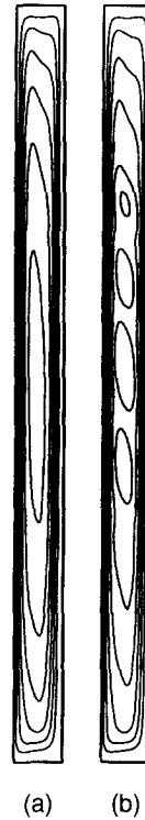
Fig. 5. Typical flow patterns at 90% glycerine-water solution with \psi = -6, -12, -18, -24, -30 and -36 \times 10^{-5} : (a) Gr = 450 ; (b) Gr = 500 .
