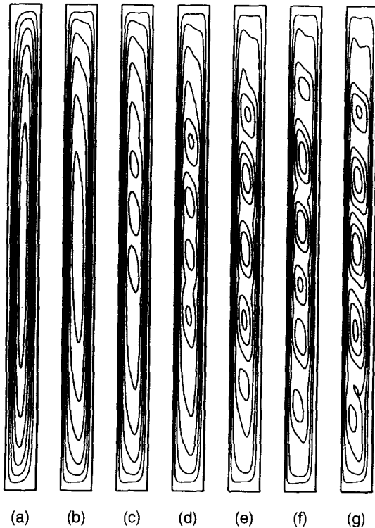
Fig. 1. Typical flow patterns at 80% glycerine-water solution: (a) Gr = 50 , \psi = -28, -56, -84, -112, -140 and -168 \times 10^{-5} ; (b) Gr = 800 , \psi = -6, -12, -18, -24, -30 and -35 \times 10^{-5} ; (c) Gr = 850 , \psi = -6, -12, -18, -24, -30 and -36 \times 10^{-5} ; (d) Gr = 1000 , \psi = -6, -12, -18, -24, -30 and -35 \times 10^{-5} ; (e) Gr = 1200 , \psi = -6, -12, -19, -25, -30 and -34 \times 10^{-5} ; (f) Gr = 1500 , \psi = -5, -10, -16, -22, -27 and -31 \times 10^{-5} ; (g) Gr = 2000 , \psi = -5, -10, -15, -20, -25 and -29 \times 10^{-5} .
